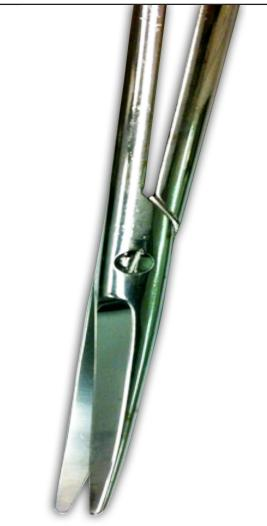
*Photo 6: Surgical scissors from*1954, *high polished surface (courtesy of Stille AB)*
