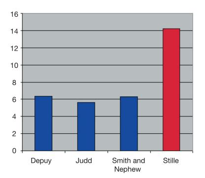
The diagram indicates the depth of cut (mm) achieved in 60 seconds. Ten test pieces were fixed onto a mechanical test apparatus and the mean depth achieved was calculated. Results of this study indicate that the Stille Gigli saw was more than twice as effective in removing material than any other brand in the study.
